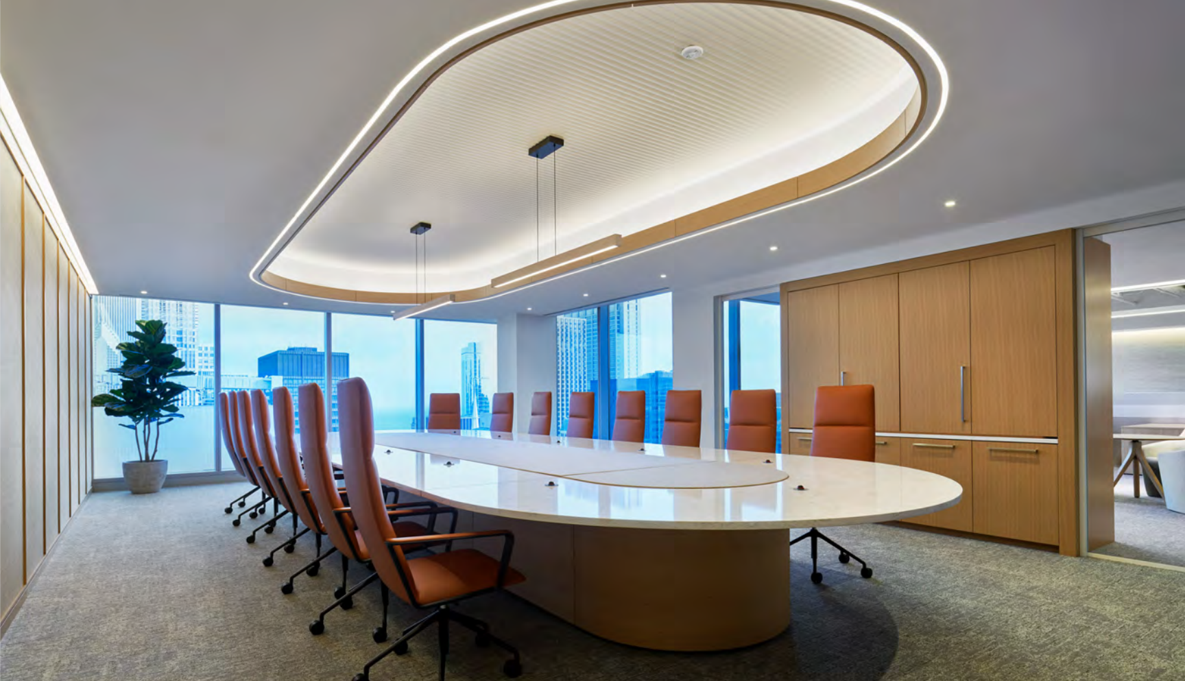
Pill-shaped boardroom table: CNC'd quartz top + fabric infill panels + oak veneer panel drum base + power integration Charlie Greene Studio
