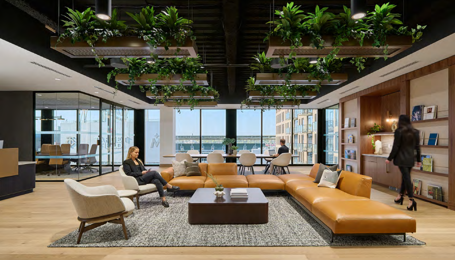
Rectangle ceiling elements: steel tube + expanded metal mesh infill + custom color powdercoat ESG Architecture & Design
