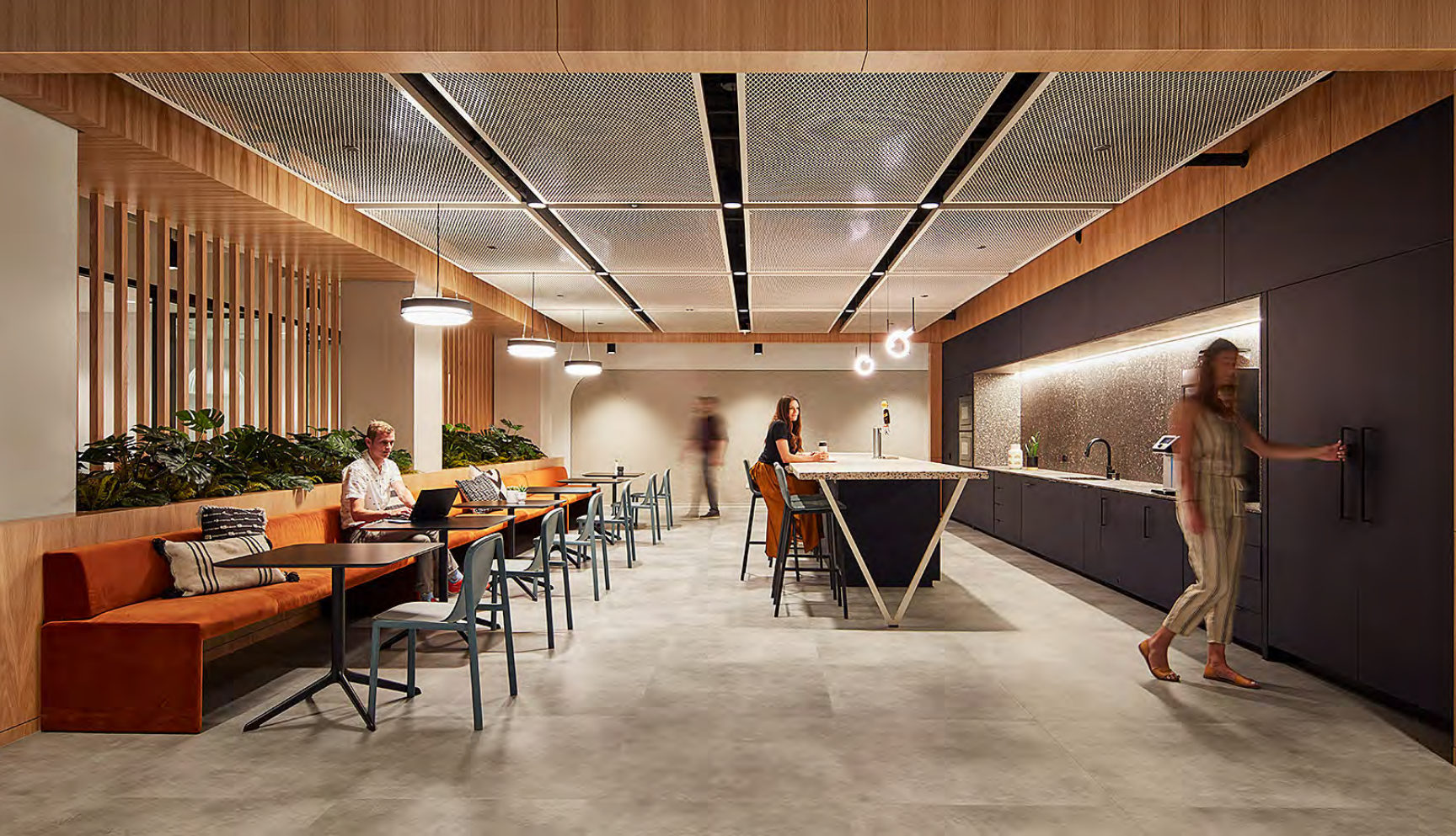
Steel tube + expanded metal ceiling panels + custom color powdercoat Partners by Design
