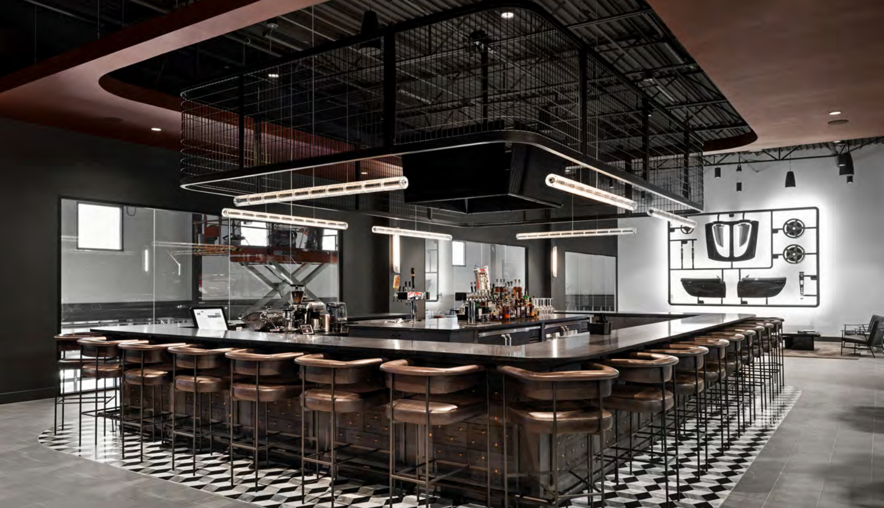
Steel tube frame with radiused corners + wire mesh infill Studio M
